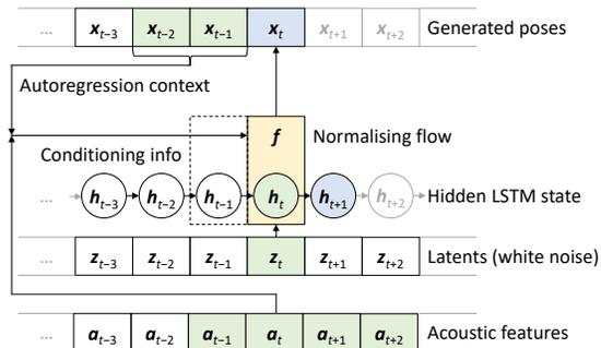
Figure 1: System overview. Green elements are inputs, blue outputs.
