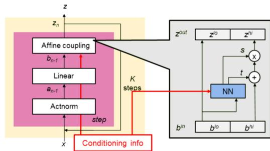
Figure 2: Structure of the normalising flow during inference. During synthesis the arrows are reversed.
